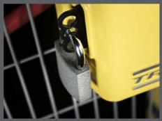
A padlock can be used to prevent the door from being locked during maintenance operations.
