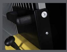
Mount a blind rivet to prevent the Safe Lock from being defeated.
