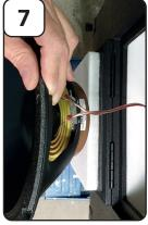
Disconnect the speaker by pulling off the terminal connections.
