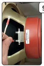
Connect the cable. One of the cables has a red line, this is your + The speaker also has a clear marking for + and -
