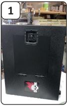
Disconnect en remove the microphones, and turn the unit on the left side.
