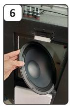
You can now take out the speaker by tilting it slightly, it will easily fit (diagonally) through the opening.
