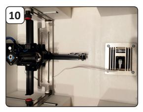
Put the BoD back on its wheels, connect the cable to Dynamount, slide in the speaker and you are ready to use the Dynamount.
