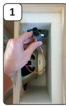
Disconnect en remove the speaker and remove microphones.
