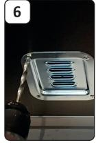
Gently place the BoD on its side, put a piece of paper on the floor (to collect the iron filings) and use a drill (Ø6mm or bigger) to drill out the cap of the rivets.
