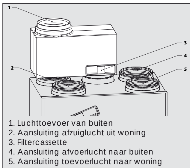
Figuur 4.2. AirMaster bypass
