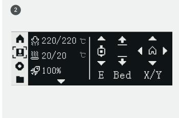
Select " $\square$ "-" $\square$ ", and heat the nozzle to the recommended temperature for the filament. Select " $\square$ "-" $\square$ " several times until the filament comes out from the nozzle and cannot be pulled out from the PTFE tube anchor manually.
