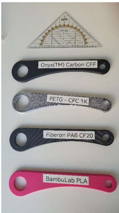
Figure 2: Plastic components in their initial state (left) and after the tensile test, front and rear (center, right)
