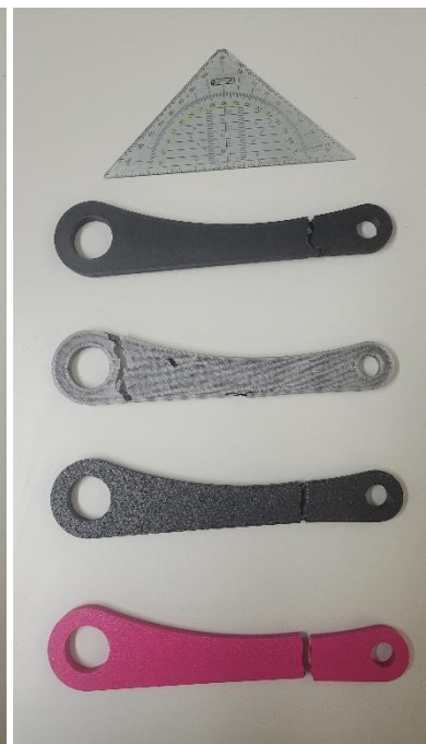
Figure 2: Plastic components in their initial state (left) and after the tensile test, front and rear (center, right)
