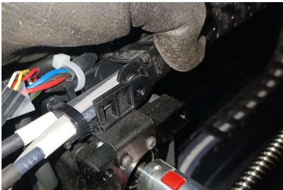
Figure 13 Disconnecting cable chain
