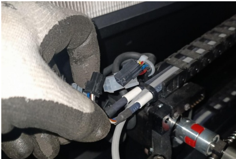
Figure 12 Disconnecting X motor cables
