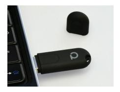
The ConBee II from dresden elektronik is a USB version of the popular and individual gateway solution for ZigBee networks. The special feature of this solution is the inconspicuous USB format, which is ideal for the operation on Mini-PCs or Raspberry Pis.
