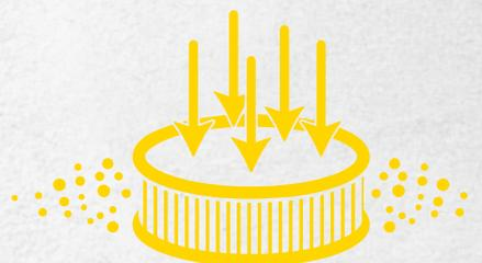
Pushing (or pulling) some times the lateral flap and closing the suction intake at the same time, it is possible to get an immediate filter cleaning, thanks to the differential pressure generated. This simple operation guarantees the maximum filtration capacity and best vacuum cleaner performance.
