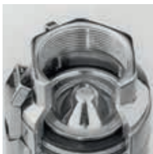
Delivery connection point in microcast AISI 304 stainless steel with an internal tapered double profile with a stainless steel non return valve and a double slot for safety cable.
