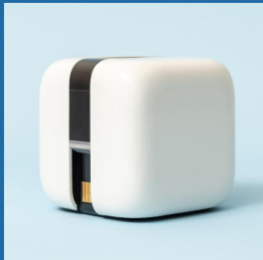
**6-7** Slide Print Cartridge in and click into place. Replace Ink Cover on the printer.
