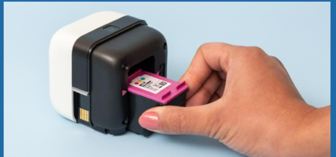
**5** Align purple cover on the top of the Print Cartridge with the purple arrows. Your Printhead will be facing the bottom.
