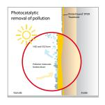
Thanks to the product's water- and oil-repellent properties, dirt cannot cling to the surface and is washed off by the rain. Surfaces treated with ProtectGuard<sup>®</sup> Dtox thus become self-cleaning.
