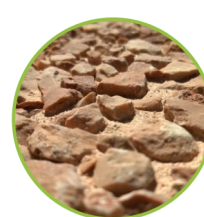
Deep exposure. Exposure depth approx. 6 mm
