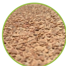
Micro exposure. Exposure depth approx. 1.5 mm
