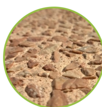
Medium exposure. Exposure depth approx. 2.5 mm
