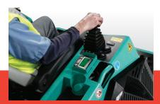
**Proportional hydraulic steering** and joystick controls allow precision performance with minimal effort, preventing operator fatigue.
