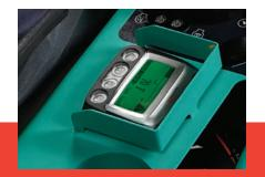
**Multifunction display** provides operator with easy-to-read data including engine speed, fuel levels and alerts.
