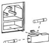
Step 1: Open the fuse holder on the rear panel with a fitting screwdriver.
