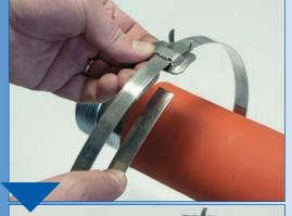
Pull buckle on band, ears pointing towards end of band. Form clamp, holding band on band, then push buckle back over the doubled band, bending the end approx. 1" under buckle.
