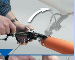
Place band in tool, push down on gripper with thumb, tension clamp by turning handle. Maximum tension is reached when band stops moving through buckle. When required tension has been applied, roll tool over buckle, at the same time reversing handle carefully approx. ½ turn to avoid breakage. There is no loss of tension, if handle is not reversed too much.
