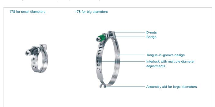
Choice of engagement positions: clamp can be adjusted to several different nominal diameters Narrow Band: concentrated transmission of clamping force, complies with SAE J1508 Type SSPC 360° StepLess<sup>®</sup>: uniform 360° compression and constant surface pressure Burr-free strip edges: reduced risk of damage to the part being clamped Self-tensioning: compensates for thermal cycle diameter changes
