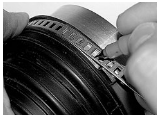
Step 2 Determine the clamp length.
