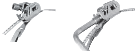
Tighten the clamp with a 5 A/F hexagon wrench. This system may not be entirely suitable for soft and flexible components.
