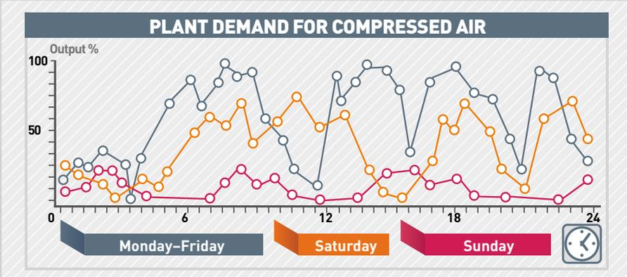
Conventional screw compressors are not able to switch between operating modes according to a plant's current demand for compressed air. Owing to constant switching between loading/unloading modes or the idle running of compressors, conventional screw compressors consume consistently large amounts of electrical energy when operating. The Comprag AV compressor series with frequency control has been created for economical compressor operation where there is varying demand.
