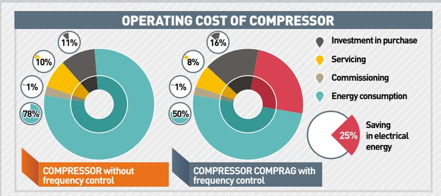
AV compressors are provided with a frequency converter for continuous control of compressor output according to the current demand for compressed air. They provide a plant with the necessary amount of compressed air at a given moment and at a constant set pressure, while consuming only as much electrical energy as there is demand for compressed air. This mode of operation conserves as much energy as possible.
