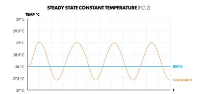
Stable output (supply) temperature, during dehumidification at night or day with the PRO4 the output temperature can go up as high as 40°C and as low as 10°C depending on the indoor temperature during dehumidification.
