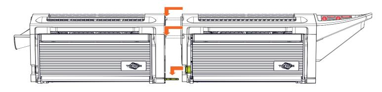
When linking more than two machines, remove the chute, belt cover and hopper from middle machine(s)
