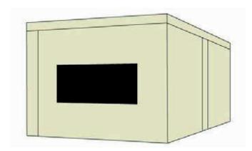
Rather cleverly the OptiClimate System can be adjusted to account for the shape of your grow room. The standard set up suits a wide area but the air outlet is actually re-positionable, allowing you to move it to the short side of the unit if you have a narrow space.
