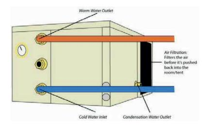
As has been previously mentioned, the unit also dehumidifies the air during the cooling process. Moisture extracted from the air enters the condensation drain, which you connect to a pipe that either feeds into your main drain, nutrient tank or humidifier reservoir. The RO water (completely purified, containing no trace elements) is suitable for use straight out of the OptiClimate System, but you may need a condensation pump to direct it to the chosen destination.
