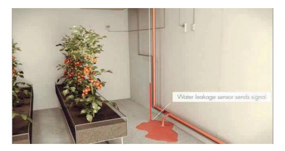
Finally, there is the option to use an excellent alarm system that notifies you of any issues and saves these message for referencing at a later date. You'll receive an SMS alert to your phone upon detection of a fault (excessive heat or a leak) and this will then be recorded by the Alarm Log function.
