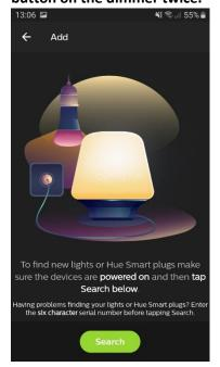
In case the app cannot find the device, push and hold the reset button on the ECO-DIM.07 led dimmer for 10 seconds. The led indicator will stay in red. Then repeat the steps as mentioned above.
