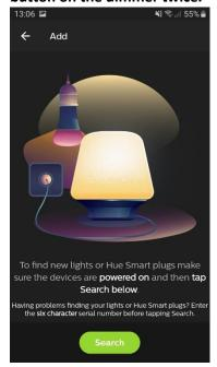
In case the app cannot find the device, push and hold the reset button on the ECO-DIM.10 led dimmer for 10 seconds. The led indicator will stay in red. Then repeat the steps as mentioned above.
