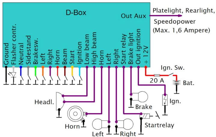
**Push button or switch input for the direction indicators (purple and orange):** You can use these inputs for push buttons or a switch what will connect the input to ground / chassis when pressed. An closed contact will start the indicator. These inputs can also be use for the **2 – Button Mode (Option 6)**.
