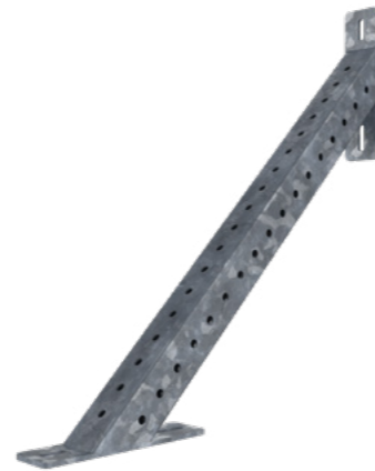
LMX1962 Crossmaxx® Outdoor Diagonal Length: 780mm | Tube size 80x80mm | Galvanized
