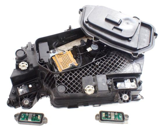
The original emitters are removed from the heatsinks, and the new are mounted. Remember thermal paste. Notice the arrows where you can bend the wings, so that they clamp on the taps of the heat sink.
