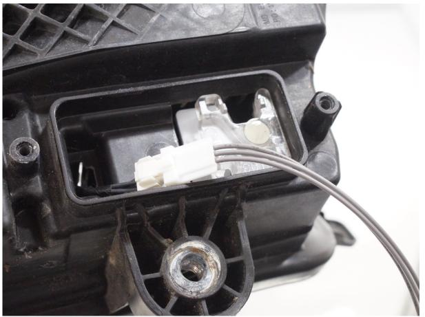
The two cables are connected to the outer connectors on the controller. Again, notice that there are two different connectors, 2-wire and 3-wire.
