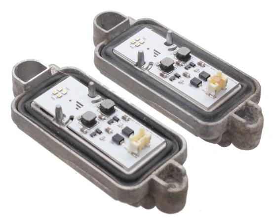
The large white male-connectors that are included, must be connected to the cables where the original emitters were connected. Notice one is 2-wire, the other is 3-wire. Cables and connecters must be fed through backwards into the headlight, this is done the easiest by pushing the cables a bit in, and catch them on the backside with fingers or pliers.
