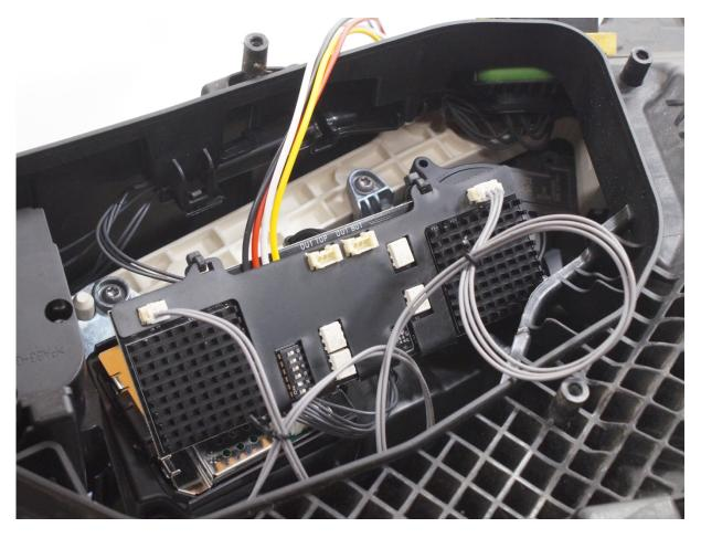
The two included female-female cables are connected to the dual color emitters, and the cables are fed through the holes into the inside of the headlight.
