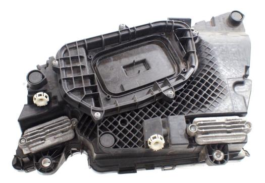
You do not have to remove the headlight completely, but you will have to tip the cabin all over. Remove the large plastic-shield and the two aluminium heat sinks, where the emitters are placed. Disconnect the connectors from the emitters.
