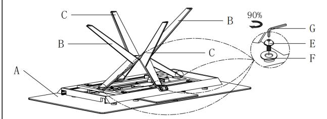
2.Please assemble the connector (D) to the corresponding position at the middle of leg frame (B&C) with bolts (E) by allen key (G);Fix the bolts for 90%;
