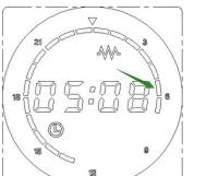
For example: the current time is 05:08, shown as green arrow \_\_\_\_\_, on for 3 seconds and off for 1 second.
