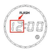
4. 5. 2. After the hour setting, short press . Then the minute position "00" will flash (flash every 0.5S). Short press or to adjust the minute with adjustment range of 0~59min. Each short press stands for 1min. Long press or for 1s can
