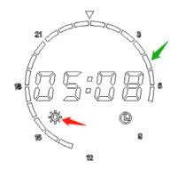
4. 6. Child lock: press and for 3s at the same time will enter the child lock. No operation allowed under child lock mode (except on/off switch). Press and for 3s
