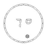
In antifreeze mode, a short press will switch to timing mode.
