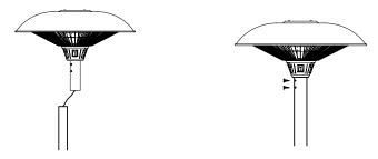
Step 5: Pull the power cord gently out of the base as much as possible. Fix the power cord under the weighted base using the supplied 4pcs M4 nuts.
