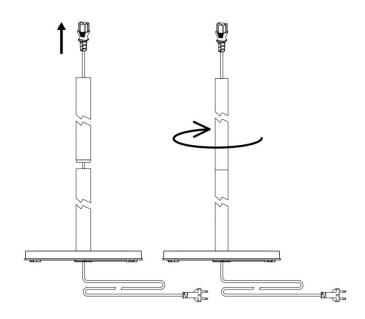
Step 3: Place the power cord plug through the upper steel pipe and connect the top tube with middle tube by screwing them together (as same as Step2).
