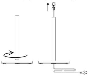
Step 2: Place the power cord plug through the middle steel pipe and connect the middle tube with bottom tube by screwing them together.
