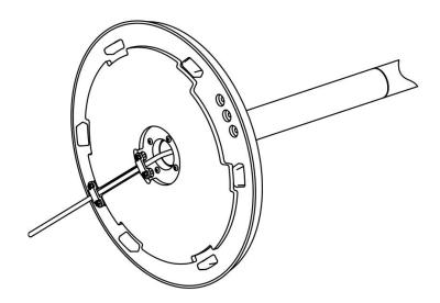
Step 7: Fix the heater on the floor. Bore three holes in the floor, fix the heater by three wedge bolts on the floor tightening the screws by spanner.
