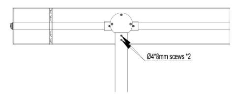
Step 6: Fix the Power Cord on the Base by using the 4\*M4 screws.
