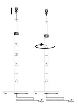
Step 4: Connect the power cord plug to the socket in the heater head.
