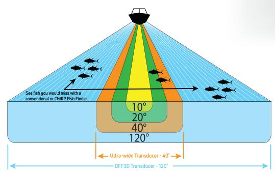
The DFF-3D Multi Beam Sonar operates at 165kHz, giving you fantastic depth penetration while still displaying echoes in high-resolution. Compared to a 40° ultra-wide transducer, you will see 3-times the area around your boat, helping you to find fish you might have otherwise missed. Plus, you can see which side of the boat they are on!
