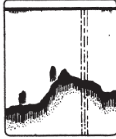
Interference from electrical equipment
