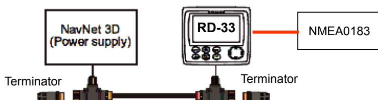
Fig.34 (b) Connection of NMEA0183 to CAN bus network with RD-33
