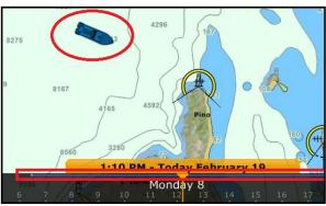
You can click on the blue boat icon (replay boat) to access the data that was recorded at that time (wind, speed, depth etc.).
