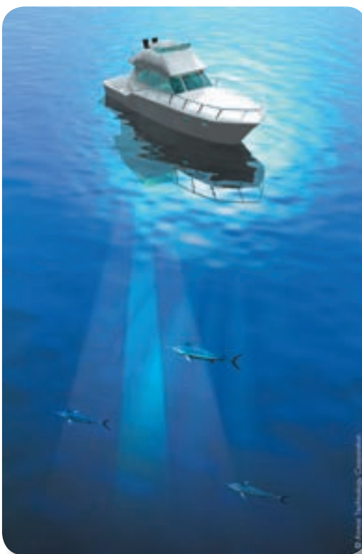
This image demonstrates the difference in beamwidth of 50kHz and 200kHz. In this example, the wider 50kHz beam will show returns for fish that the narrow 200kHz beam would have missed.
