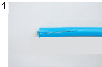
Expose inner vinyl sheath.
