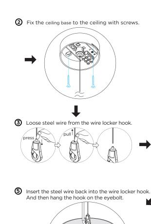
strain relief . 6 strain relief Let the steel wire through the rubber rings that attached on the cable. steel wire shade cable rubber ring (8)
