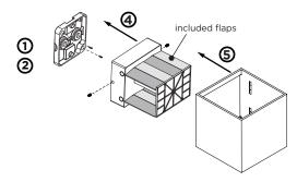
with flaps, the beam angle is adjustable:
