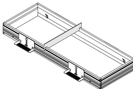
Now you can insert the plaster kit into the hole in the ceiling.
