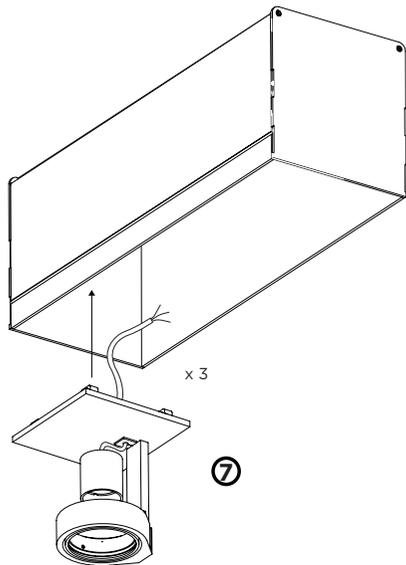
Insert each fixture into the recessed housing.
