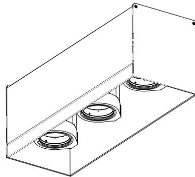
Insert the PAR16 lamps (If you have the LED version, this step is not necessary).
