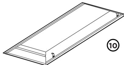
Now you can insert the recessed housing (with the connected fixtures) into the ceiling on the plaster kit but first connect the power supply to the fixtures.
