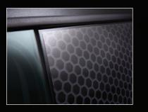
▲ Create a uniform relief cut between window graphic and rubber molding.
