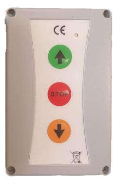
Control boardfor roller shuttersfrom 100-250V AC, with multibrand and multifrequencyreceiver RX-Multi integrated (433 MHz frequency). Up/down input switches (configurable as dead man, direct order or sequential switch). Automatic closure and photobeam signal input availables and lamp.
