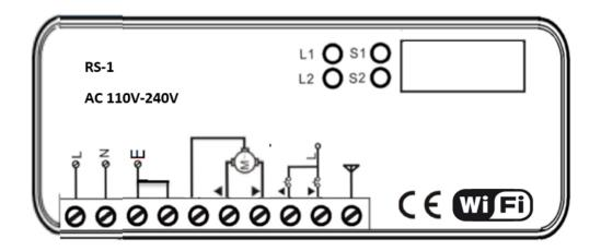
Control board for tubular motor with power supply 110 - 240 V. With function OPEN/STOP/CLOSE available for AC switch.
