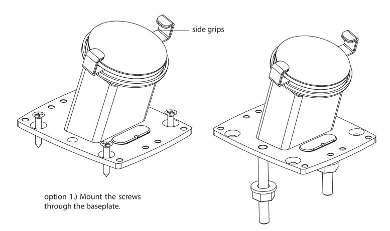
option 2.) Mount the stud/bold from underneath the display table into the baseplate. Secure with a screw / nut.
