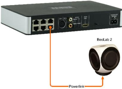
Subwoofers like a BeoLab 2 are connected to the lower right RJ45 socket.
