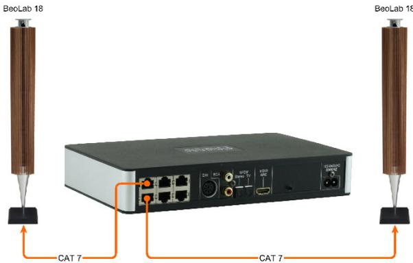
Newer B&O speakers (e.g., BeoLab 18) will be connect directly with a CAT 7 patch cable.
