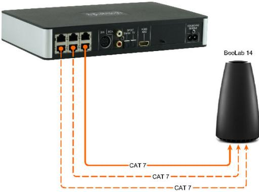
BeoLab 14 can also be connected without any problems (center and subwoofer are output separately on both audio signals of this Powerlink socket).
