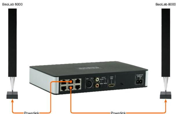
In order to connect older B&O speakers (e.g. BeoLab 5, BeoLab 8000, BeoLab 6000 etc.) you need some special adapters RJ45 <-> Powerlink.
